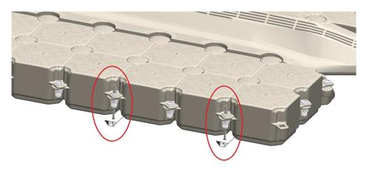
These bars are essential to ensure good stability of your Candock dock and optimum efficiency of yours Air ASSIST system. If your platform is not equipped with stabilizer bar, please refer to your Candock distributor.
